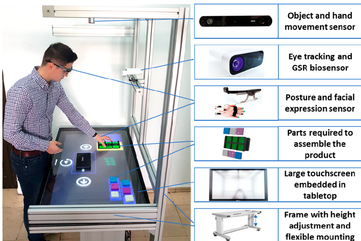
Figure 1. Assembly assistance system.
