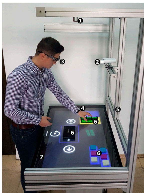
Figure 1. Manual assembly assistance system. 1: Depth camera for object detection; 2: facial expression and posture recognition sensor; 3: eye-tracking glasses; 4: GSR sensor; 5: height adjustable frame; 6: different parts of the assembled object; 7: large touchscreen.
