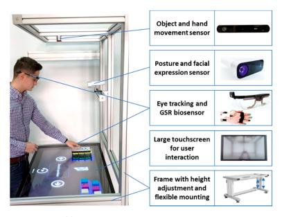
Figure 1. Assembly assistance system.
