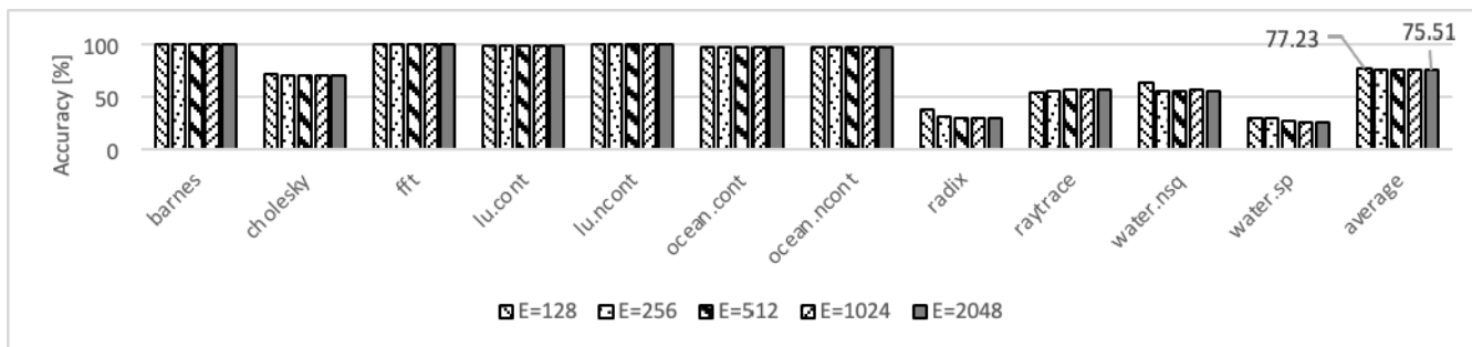
Figure 3. Averaged prediction accuracy per core for all benchmarks by varying number of entries ( E = \{128, 256, 512, 1024, 2048\} ; A = 4 ; H = 4 ; C = 4 )
