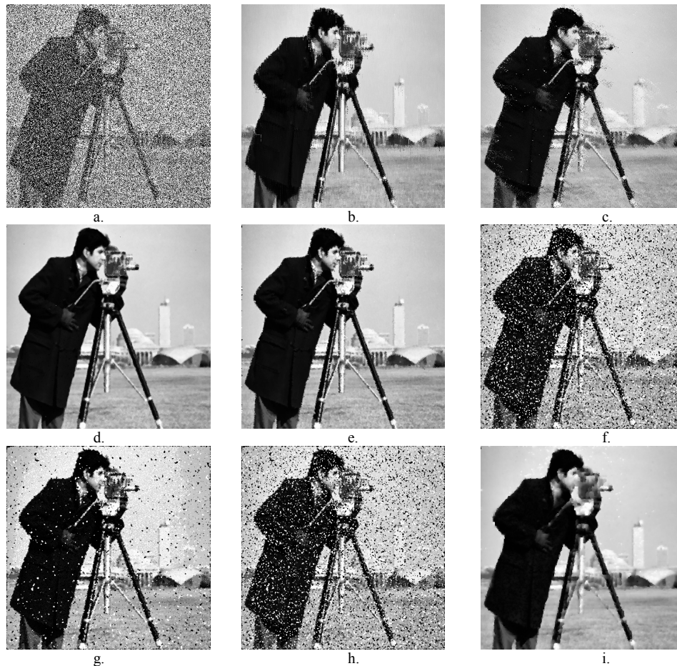
Fig. 10 Denoising the Cameraman image having 60% noise (a) using the S^*_C+ Markov filter (b), CBPF (c), NAFSM (d), DBA (e), MF (f), PSMF (g), RMF (h), APA (i)
