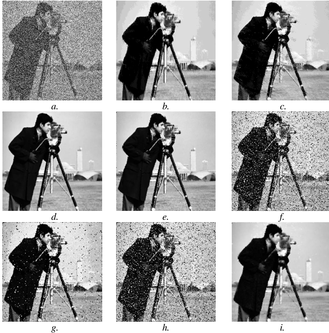
Figure 87. Denoising the Cameraman image having 60% noise (a) using the S^*_C+ Markov filter (b), S0\_C0 Markov filter (c), NAFSM (d), DBA (e), MF (f), PSMF (g), RMF (h), APA (i)
