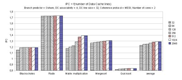
Figure 3: IPC as a function of the number of lines of the data cache from a dual-core SMP
