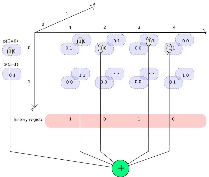
**Fig. 3.** Schematic diagram of simplified Naive Bayes predictor, calculating the likelihood that the next branch outcome will be 0 given the history 1010. The complete calculation requires checking the likelihood that the next branch will be 1, and then selecting the larger probability as the predicted outcome.
