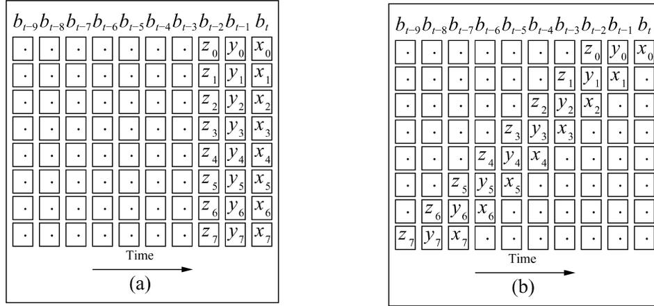
Fig. 3. Illustration of the weights used to predict branch  $b_t$  with the perceptron predictor (a) and the path-based neural predictor (b) with history length of 7. Vertical columns are weights vectors.
