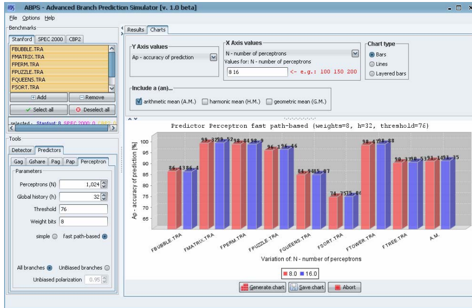
Figure 6.4. ABPS simulator – variation of prediction accuracy with global history length.
